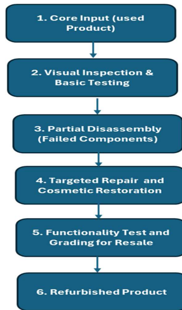
Fig 2. Refurbishment Process Flow – Selective Restoration Approach.
