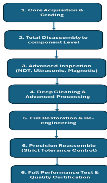
Fig 3. Remanufacturing Process Flow – Zero-Fatigue Reconstruction Approach.
